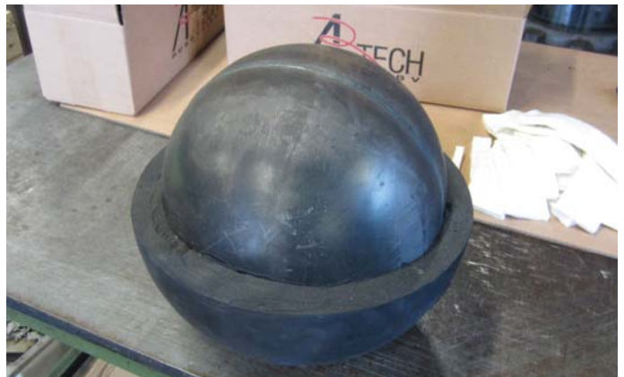
Once encased on rubber, metal balls like this are used in non-return valves on pipelines. By allowing air into the pipeline the valves help prevent compression damage.
