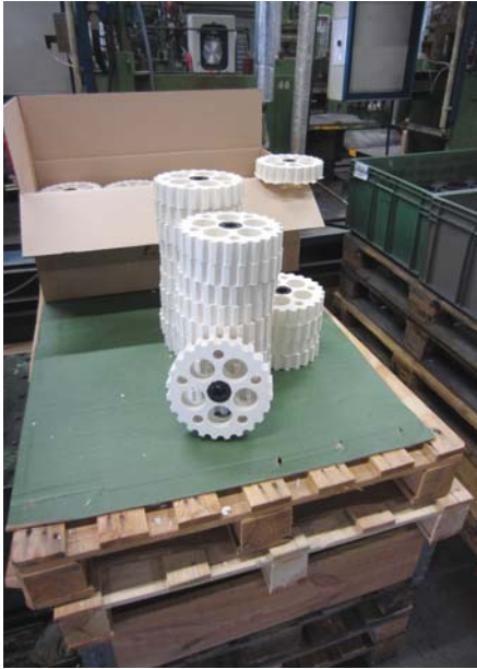
This two-component ring has a soft rubber inner ring with a hard plastic lining and is used for transport systems in the food industry.
